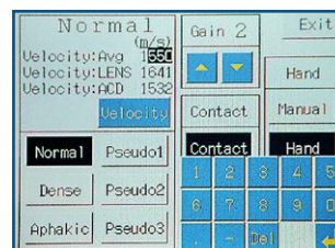
The AL-100 provides full access to ultrasound velocities
